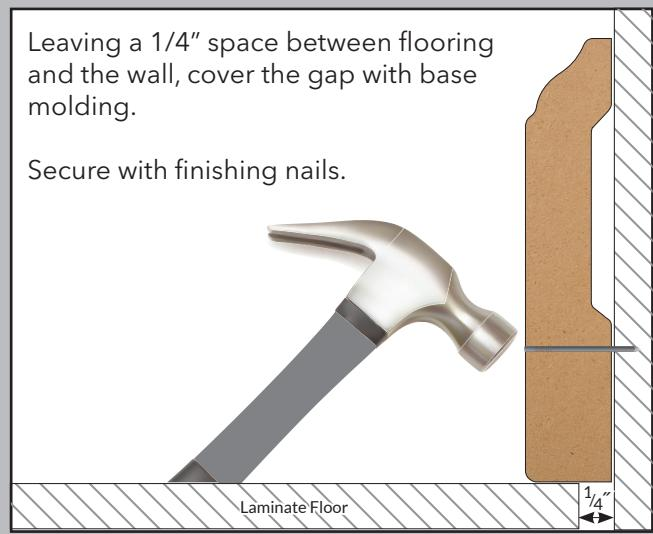
Leaving a 1/4" space between flooring and the wall, cover the gap with base molding.
