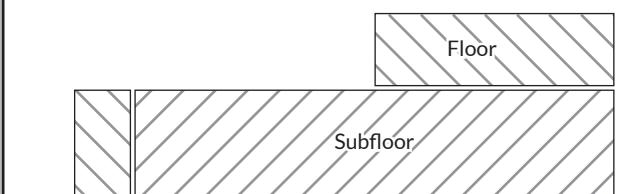
Install the flooring leaving a 1-1/4" space from the end of the step for the stair nose installation.
