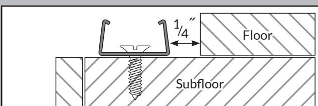
Position the track 1/4" from the floor plank and screw to the subfloor using included screws.
