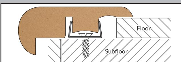
Starting at one end, press the molding into the track inching along the length of the molding. It will NOT snap in all at once. You may also use a rubber mallet.
